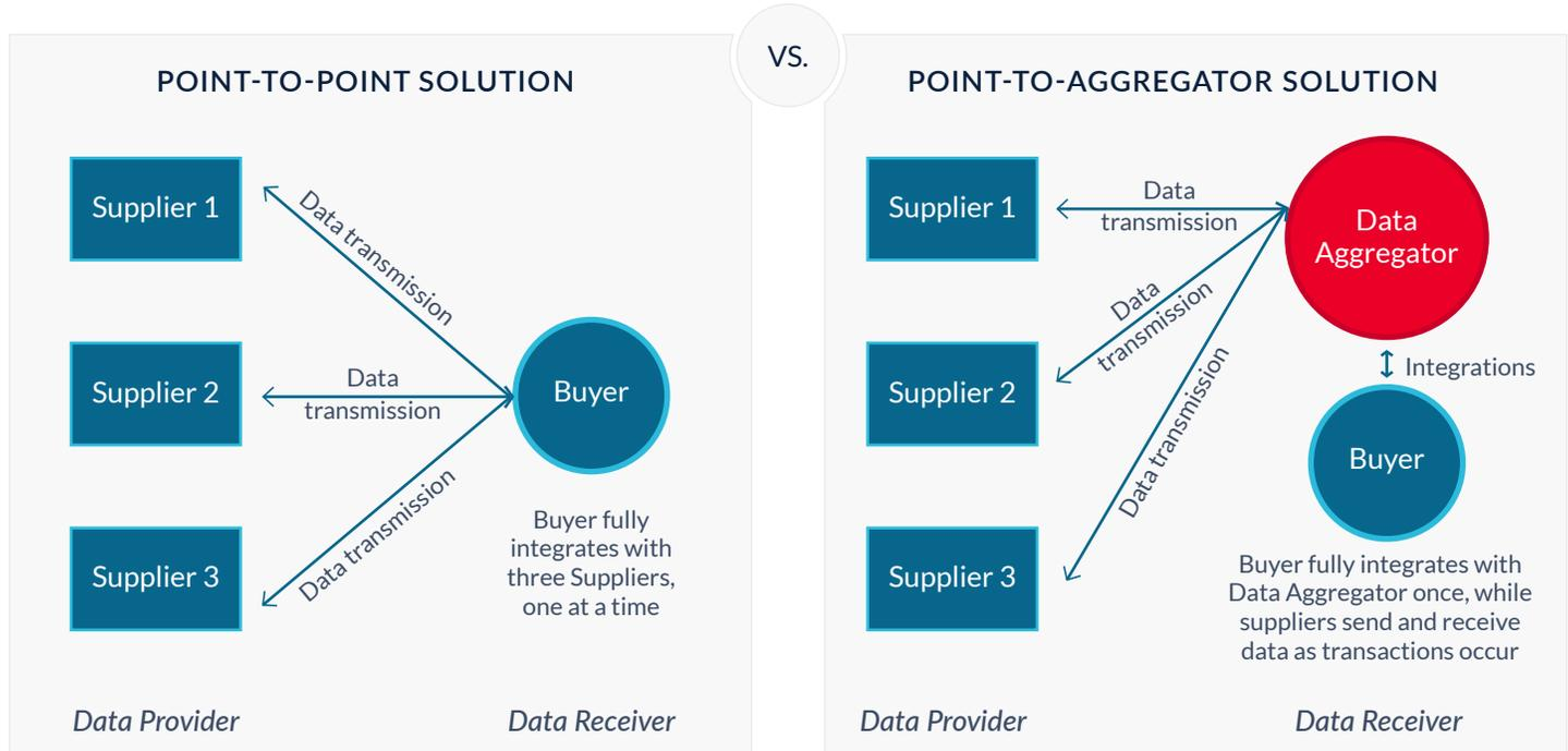
**FIGURE 1** Comparison between point-to-point and point-to-aggregation solutions
